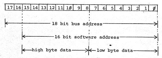
The processor converts the software address to a full 18-bit bus address. On word bus commands (DATI, DATO, DATM), the slave ignores DØ; on byte bus commands (DATOB, DATMB), slave receives byte data on D (15:8) if DØ=1 or D (7:0) if DØ=0.
